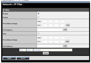
The IP Filter setting allows the administrator of the camera to limit the users within a certain range of IP addresses to access the camera.
